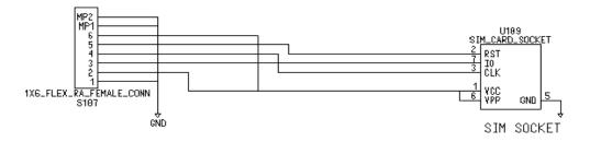
SIM Interface and Test Board integration
