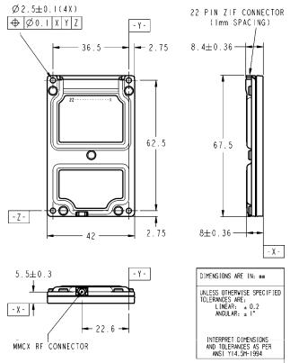
MOUNTING HOLE PATTERN: 4 HOLES IN A 62.5x36.5mm RECTANGLE.
