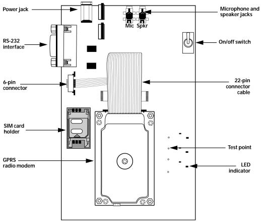
Interface and Test Board for off-board configuration- top view
